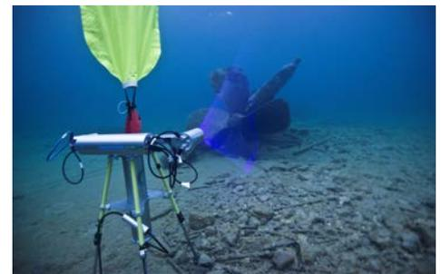
Above/Below, laser scanning the steamer *Monohansett's* stern. The unit was moved incrementally around the wreck to create a 3D point cloud model of the wreck site.
