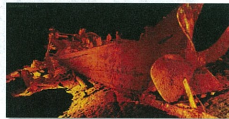
Above/Below, laser scanning the steamer Monohansett 's stern. The unit was moved incrementally around the wreck to create a 3D point cloud model of the wreck site.
